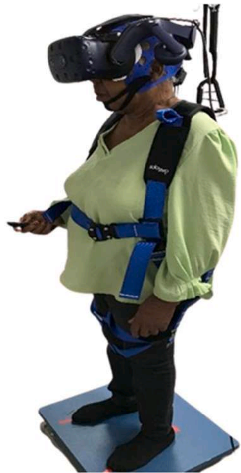
Fig. 1. Experimental setup of the standing condition. Participants completed quiet standing (condition 1) of the Virtual Reality Sensory Organization Test (VR-SOT) using the Virtual Reality Comprehensive Balance Assessment and Training (VR-COMBAT) system (Participant is bending the right elbow for demonstration purposes to show the clicker). Participant signed photo and video release statement.
