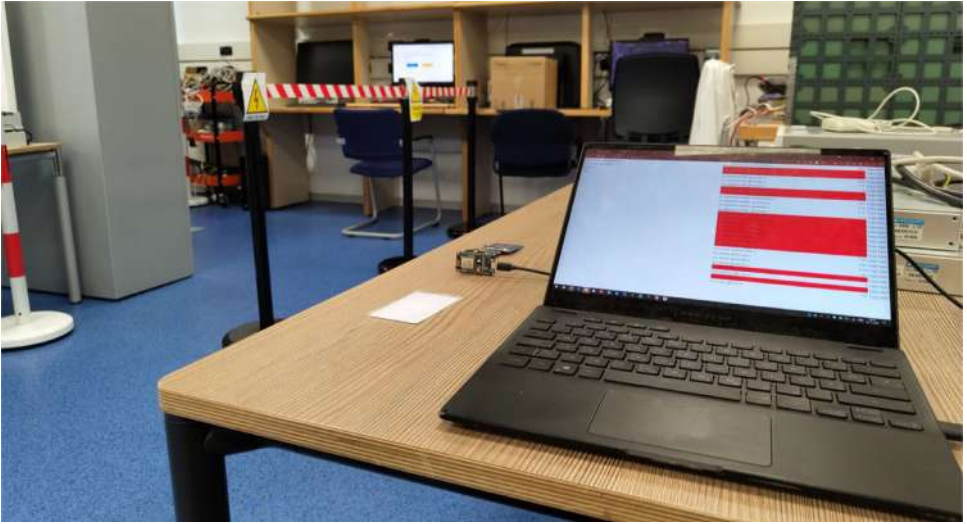
Fig. 4. An image of the experimental testbed from the perspective of the operator. The laptop on the right is running the real-time monitoring software which helps the operator to immediately spot any potential issues. Each experimental run starts here with sensor initialisation. In the background the volunteer-operated PC is shown.
