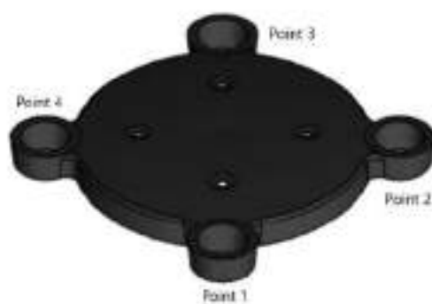
Figure B1: Grid-electrode used as an anode with measurement points numbered.
