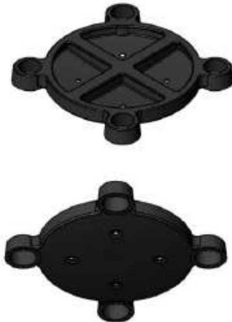
Figure 14: The figure shows a 3D model of the electrode cup used as an anode in in vivo measurements. The anode is divided into four blocks isolated from each other by a cross in the middle. In addition, locations for the measurement electrodes are placed on the outer edge of each segment. This solution aims to minimize the risk of the measurement electrode getting wet and the electrical interaction between the blocks.
